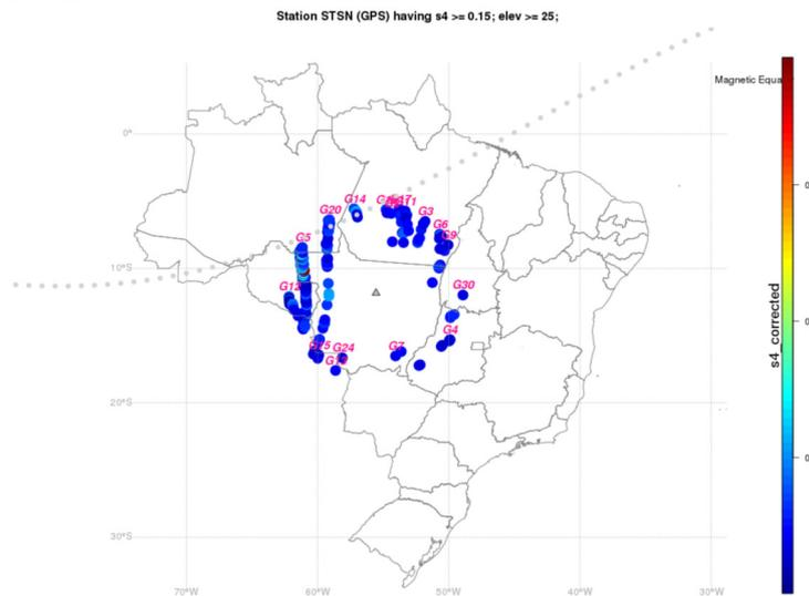
Figure 2: Map of S4 values  $> 0.15$  for GPS satellites with elevation  $> 25^\circ$  at STSN receiver field of view in between 1300-2000 UT on 07/03.
