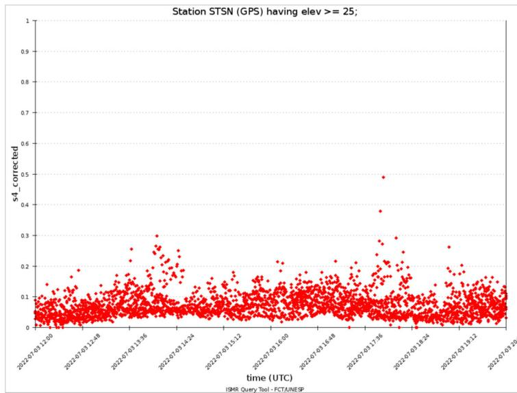
Figure 1: S4 index values for the GPS constellation measured at STSN during the morning hours of 07/03.
