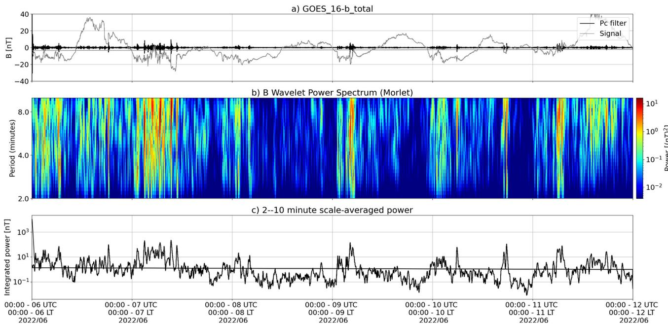
Figure 3: a) Timeseries of the geomagnetic field total component measured by GOES 16, together with the Pc5 fluctuation in black. b) Wavelet power spectrum of the filtered timeseries. c) Average ULF power in the period range from 2 to 10 minutes.
